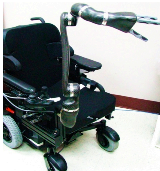
Figure 1: JACO joystick-controlled six degree-of-freedom robotic manipulator
